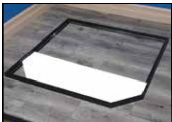
5. Lay in (1) 12" x 36" Micore 300 rectangle piece with two end cuts.
