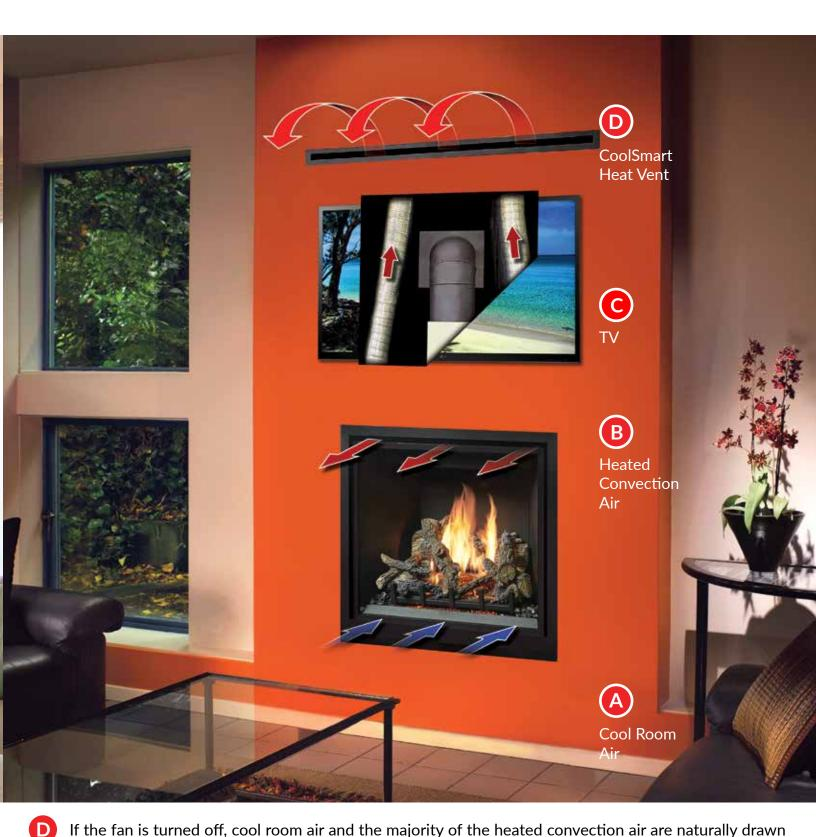
If the fan is turned off, cool room air and the majority of the heated convection air are naturally drawn up through the CoolSmart Heat Vent(s) and returned to the room above the TV. This reduces the height the TV needs to be installed above the fireplace.
