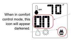
This is the comfort control read-out. Use the up button to turn on, down button to turn off (2 settings).
