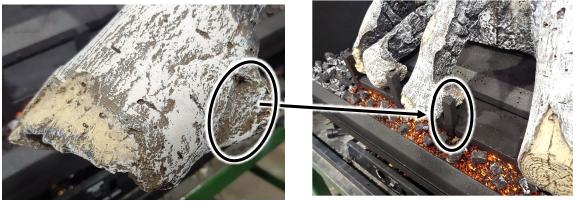
The top portion of log #8 rests against log #7. The limb on log #7 helps to lock log #8 into place (see right).
