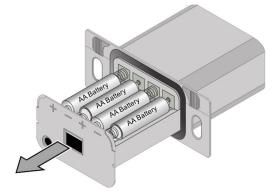
**Battery Installation**" on page 16). In applications where the appliance is required to provide heat, we recommend replacing the batteries before each heating season.
