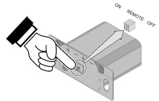
**NOTE**: When the battery holder switch is turned to ON or OFF, the mode settings (Flame Height, Comfort Control) will remain in the same state as before the switch was moved (i.e.: the IFC "remembers" the last setting). If you wish to adjust the mode settings use the transmitter mode button to adjust the settings (see "Mode Controls" on page 13). The thermostat and burner on/off operating functions will not work on the transmitter.
