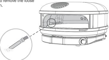
For the exterior of Arc ensure the oven is cool and use a non caustic bleach free cleaning spray on the dirty areas. Clean the area with warm soapy water and a sponge or non abrasive dish cloth and then wipe clean with paper towels. Arc's flue can also be removed for cleaning.
