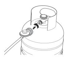
After cooking, be sure to turn off the gas from the gas canister first before turning of Arc. This will allow any gas left in the burner or pipe to be used up safely. Three minutes after turning the gas off it will be safe to remove the regulator and turn the control dial back to the off position.
