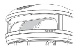
The flame should be yellow in colour and roll along the top of the oven.
